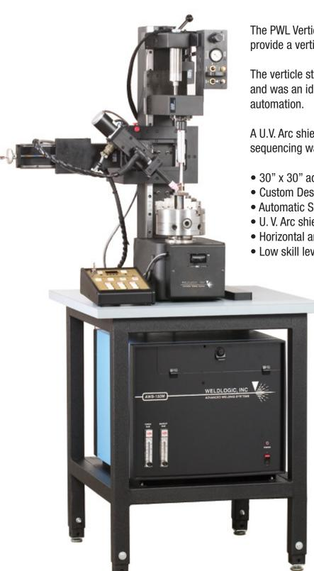
The PWL Vertical 6100 Welding System was configured to provide a verticle production welding work cell.
